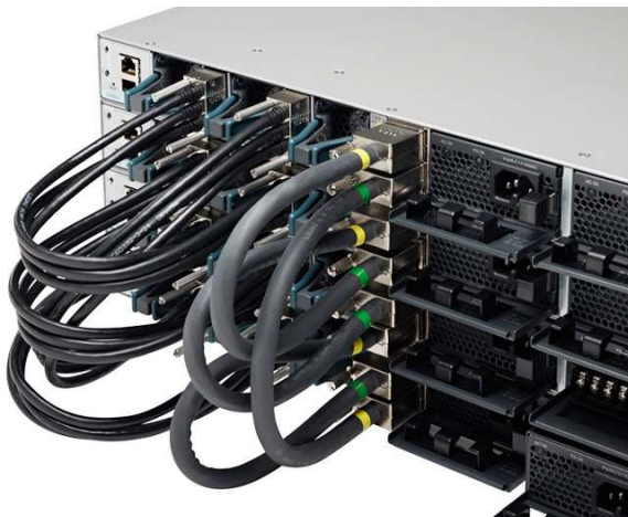
Figure 5. StackWise-480 and StackPower Connectors
